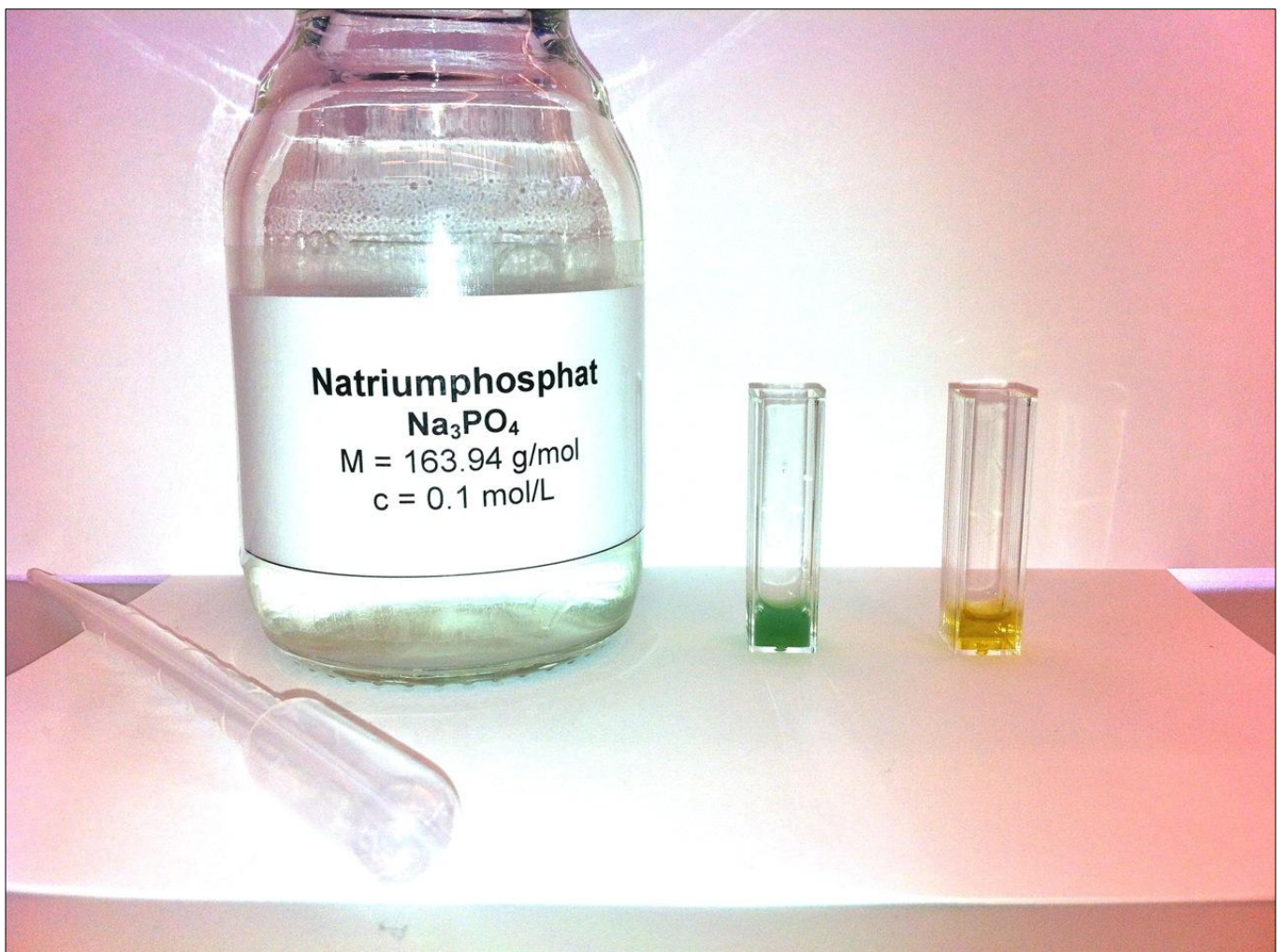
Fig. 1: The green solution with sodiumphosphate in comparison with the yellow test solution
