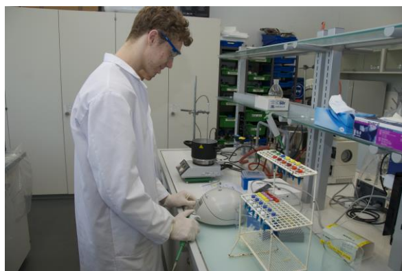
Figure 2: Centrifugation of the yeast suspension during experiment 4B. The rack in the foreground holds the EPs containing the malachite green solution and those filled with the supernatant.
