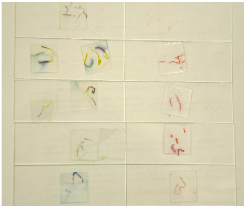
Fig.2: The very thin sections used for all of the investigations. It is visible that the soluble purple colour diffuses into the water.
